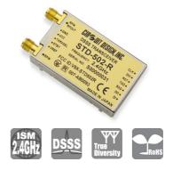
Besides using highly noise-resistant direct-sequence spread spectrum (DSSS) modulation, the module has a true diversity receiver function for preventing signal dropout due to multi-path fading. This ensures highly reliable radio communication in the congested 2.4 GHz ISM band.
